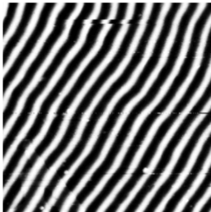
Fig. 3. Magnetic image of the 308 nm Py film ( 6\mu\text{m} scan). The half period is 220 \pm 30 nm, slightly smaller than the film thickness.
