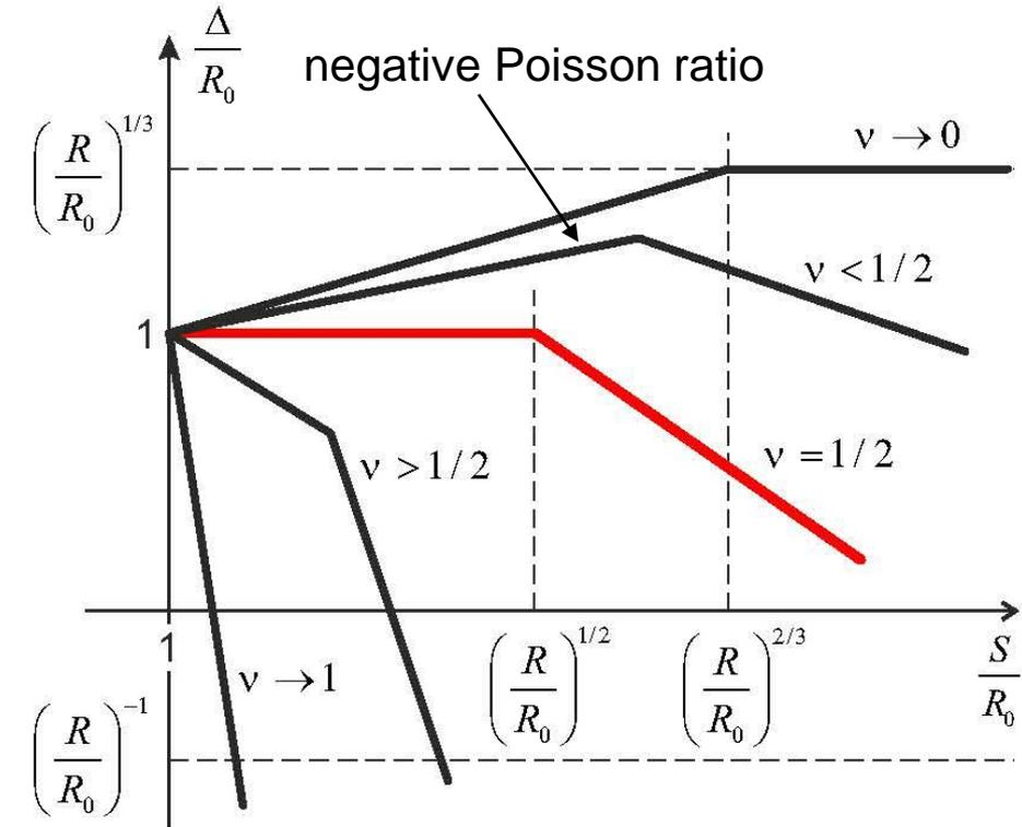
Dependence of normalized fluctuations above the disc,  $\Delta / R_0$ , on normalized chain stretching,  $S / R_0$  ( $R_0 = bN^\nu$ )
