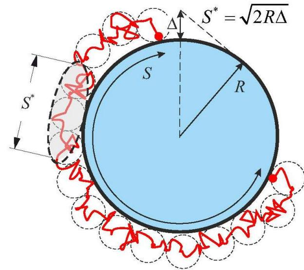
Fractal polymer ( $R_0 = bN^\nu$ ) stretching in flat tube or above impermeable disc
